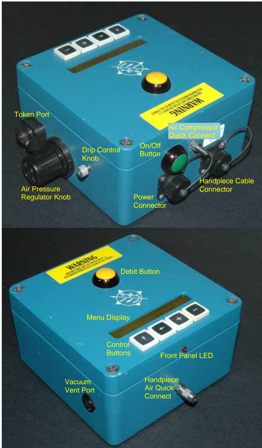
Figure 1: Control box for the Air Driven Elastomer Injection System
